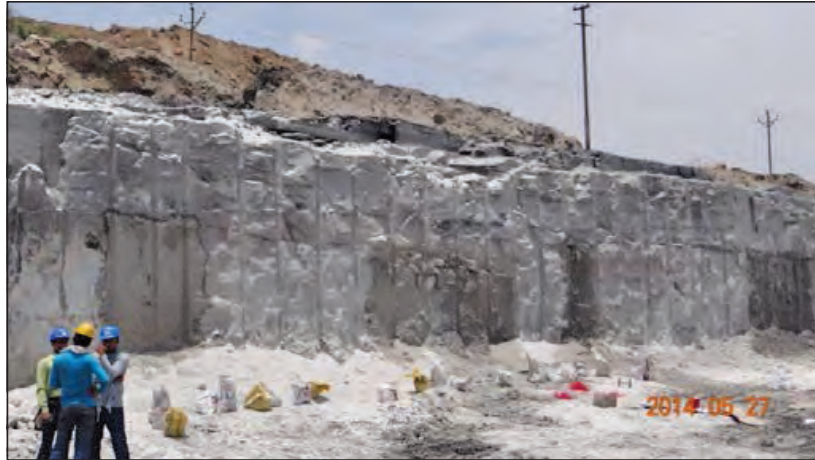
Final highwall obtained by smooth blasting at Sharda Trench Highwall Mining Project, SECL
